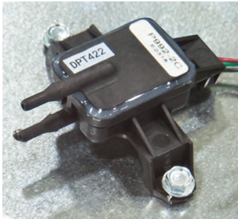
Figure 3 - Pressure Transducer in Electrical Box
