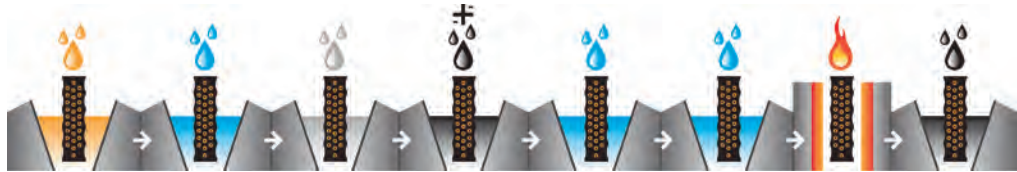
Figure 1 - ElectroFin® E-coat Process
