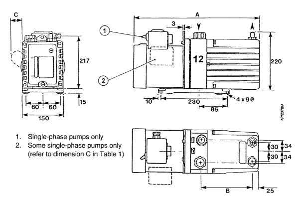
$Figure \ 5 - Dimensions \ E2M12 \ (some \ single-phase \ pumps: \ refer \ to \ Table \ 1 \ for \ applicability) \ (mm)$
