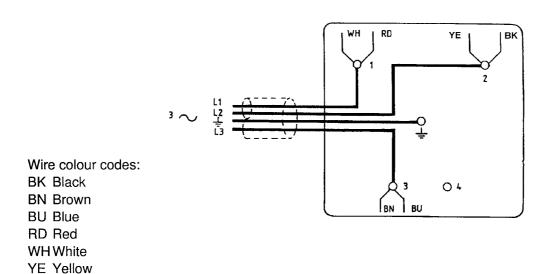
Figure 14 - Electrical supply connection, three-phase motors (low voltage) (see Table 2 for applicability)
