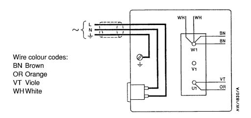
Figure 10 - Electrical supply connection, single-phase motors, (low voltage) (see Table 1 for applicability)
