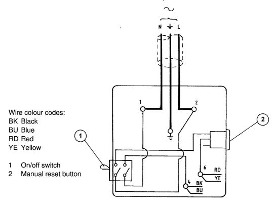
Figure 7 - Electrical supply connection, single-phase motors
