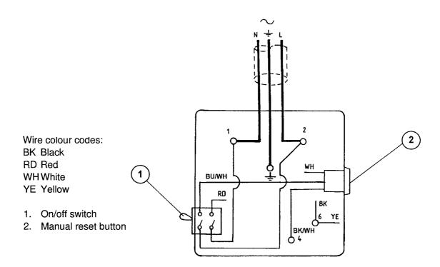
Figure 9 - Electrical supply connection, single-phase motors, (high voltage) (see Table 1 for applicability)
