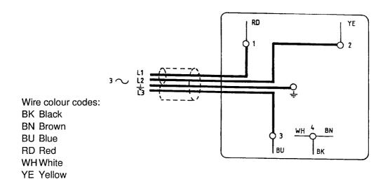
Figure 15 - Electrical supply connection, three-phase motors (high voltage) (see Table 2 for applicability)
