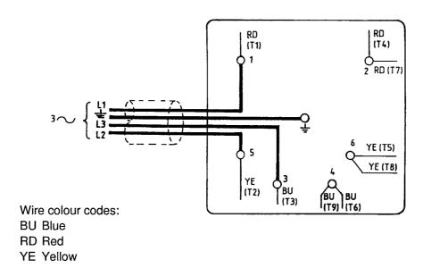
Figure 13 - Electrical supply connection, three-phase motors (high voltage) (see Table 2 for applicability)
