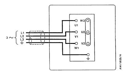
Figure 17 - Electrical supply connection, three-phase motors, ) (high voltage) 380-415 V 50 Hz, or 460 V 60 Hz, 380-420 V 50 Hz
