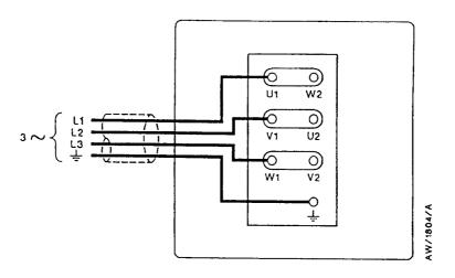
Figure 16 - Electrical supply connection, three-phase motors, (low voltage) 200-220 V 50 Hz, or 200-230 V 60 Hz 200 V 50/60 Hz, 220-240 V 50 Hz
