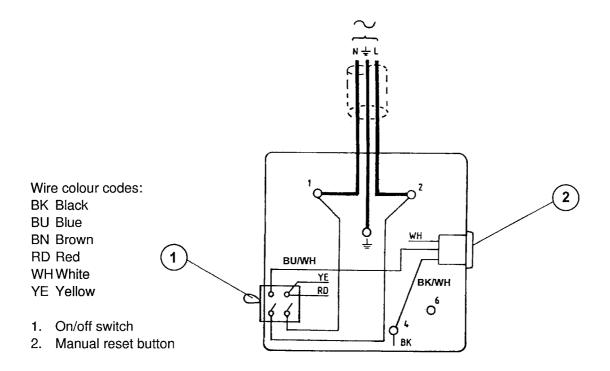
Figure 8 - Electrical supply connection, single-phase motors, (low voltage) (see Table 1 for applicability)
