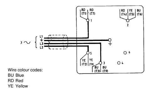
Figure 12 - Electrical supply connection, three-phase motors, (low voltage) (see Table 2 for applicability)
