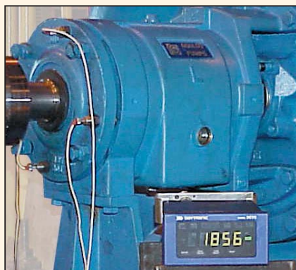
Bearing Load Measured on Test
