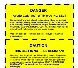
This label indicates the presence of moving conveyor belts, which may be moving through the tunnel.
