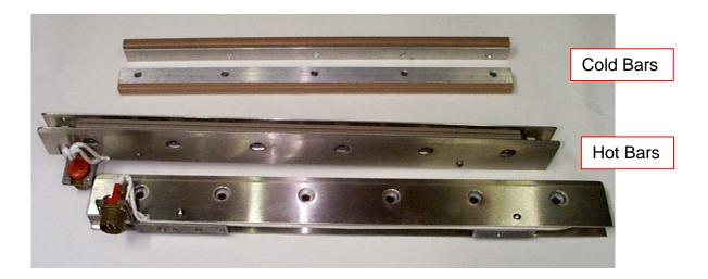
The purpose of this assembly is to seal and cut the film before and after each product. This is accomplished by squeezing two pieces of the film together between the hot and cold bars. The hot bar heats the film until the two pieces of film fuse together. Simultaneously, the knife, which is mounted in between the two Teflon coated plates, cuts the fused section of the film into two pieces.
