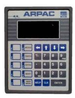
The operator uses this interface to communicate with the PLC in the machine. The screen is used to indicate the machine's current mode of operation, and any problem the machine may encounter, as well as to help the operator make any necessary changes or adjustments to timers in the program.
