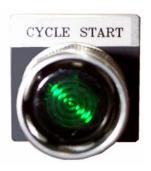
The cycle start push button starts the normal cycle of the machine.
