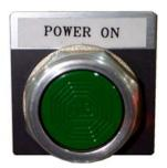
The power on push button supplies power to the main drive motor, the Mac valve, the seal bar heating element, the tunnel blowers and the tunnel heater elements.
