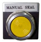
The manual seal push button will cause the seal bars to close for one cycle. This is used to splice the film together after threading the machine. This button is disabled while the machine is in the cycle and when the guard doors are open.
