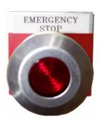
Each emergency stop push-pull button will shut down all electrical and pneumatic devices, with the exception of the controller. It is extremely important that anyone coming in contact with the machine knows where this valve is and how to use it.
