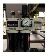
The master air supply regulator controls the air supply (typically 80 psi min.) to the machine. It is usually located on the lower control side of the wrapper. It is extremely important that anyone coming in contact with the machine knows where this valve is and how to use it.
