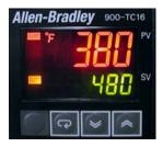
The temperature controllers control and display the temperature of the heating elements of the machine. They are labeled as to which elements they control.
