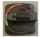
The main power disconnect supplies the main high voltage (typically 240 or 480 volts) to the machine. It is typically mounted on the main control cabinet. It is extremely important that anyone coming in contact with the machine knows where this switch is and knows how to use it.
