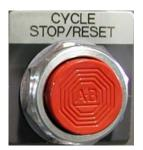
The cycle stop/reset push button is used to stop the cycle of the machine as well as to reset the controller after an emergency stop or jam situation.
