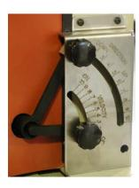
The tunnel louvers are located just above the deck at both ends of the tunnel. These adjust the direction and velocity of hot air flow to the sides of the product.
