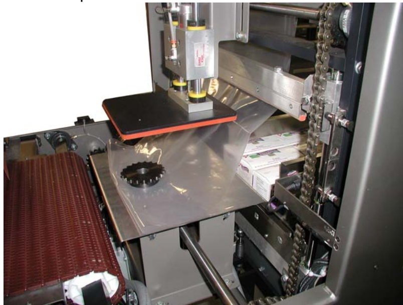
Figure 5-6. Manually Sealing Film
