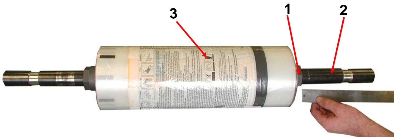
Figure 5-2. Film Roll Installation on Shaft
