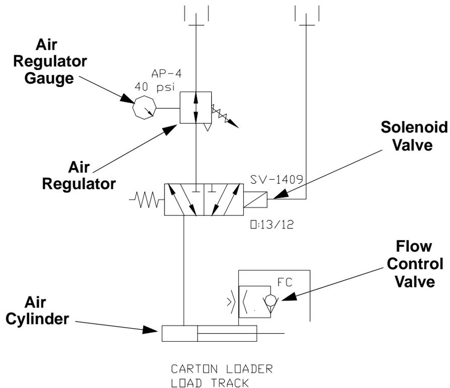
**Figure 2-19: Air Regulator and Gauge Symbols**
