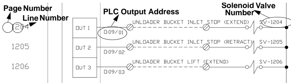
**Figure 2-3: Solenoid Valves on an Electrical Schematic**
