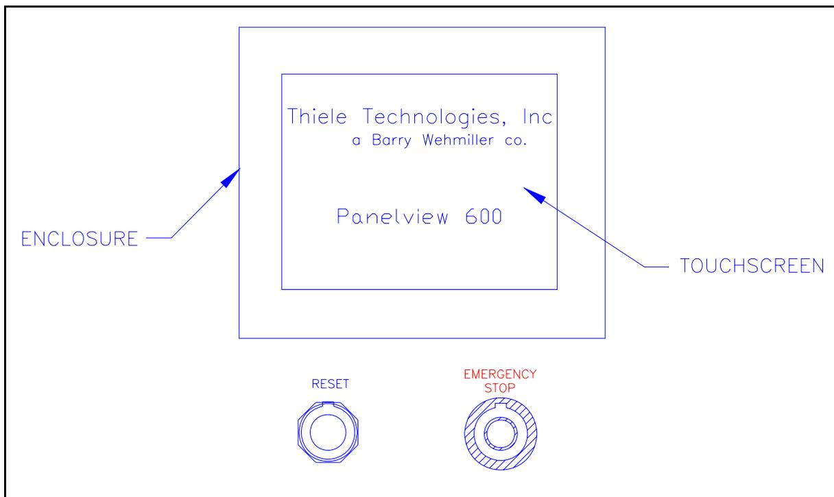
**Figure 5-1 Operator's Control Station**
