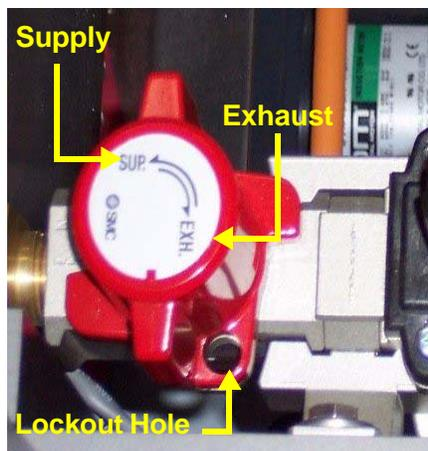
Figure 1-5 Manually Operated Valve
