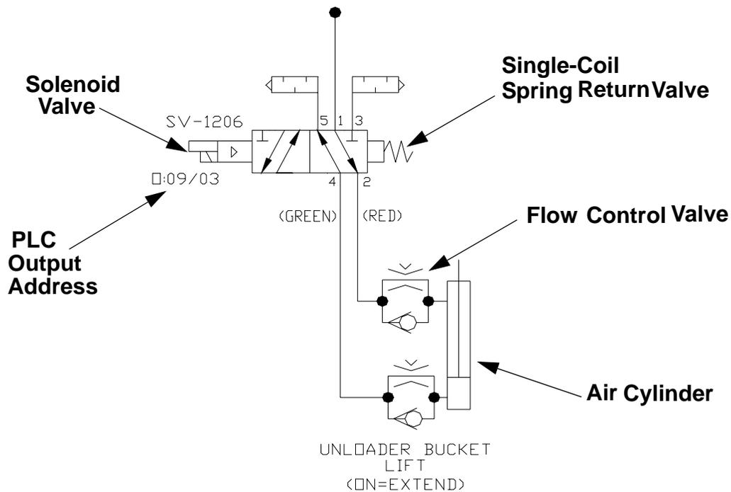
**Figure 2-6: Single Solenoid Valve on Pneumatic Drawing**
