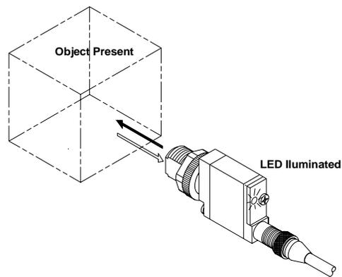
**Figure 2-15: Light-Operate Photoeye**
