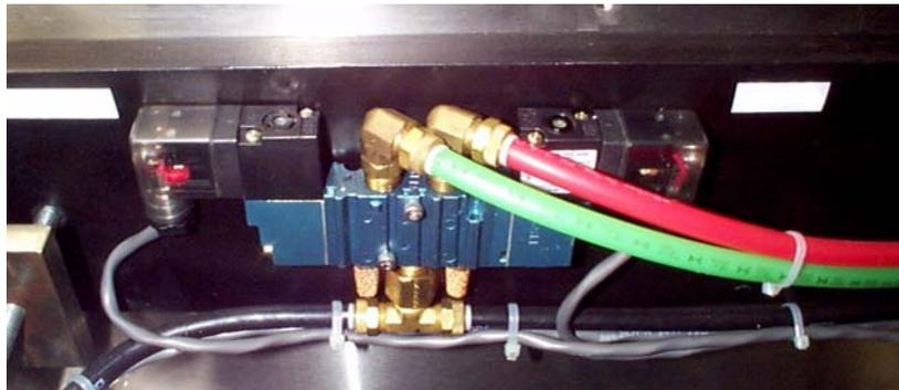
**Figure 2-7: Double Solenoid Valve**
