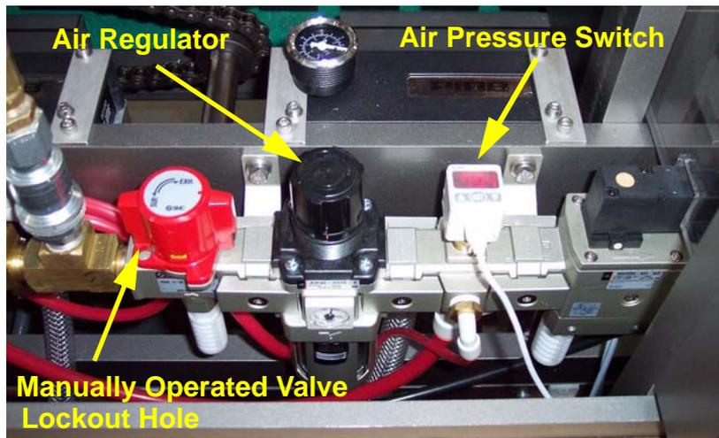
**Figure 7-1: Manually Operated Valve and Air Filter/Regulator**
