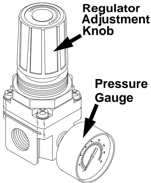
**Figure 2-18: Air Regulator and Gauge**
