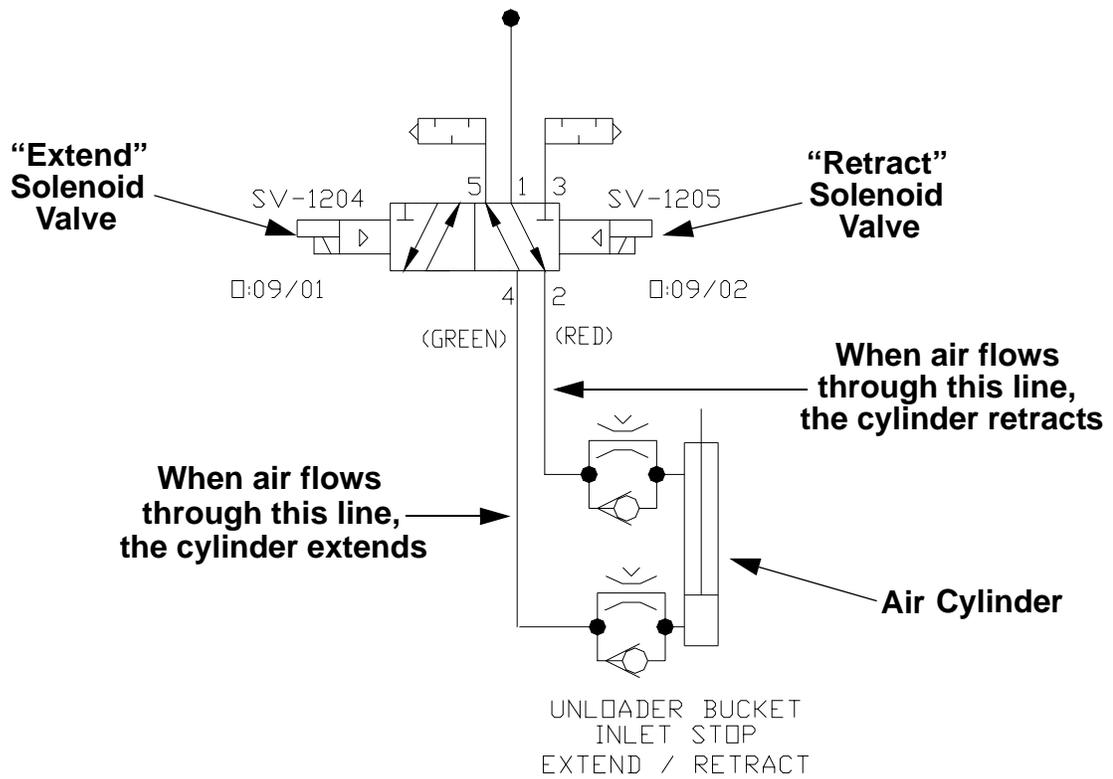
**Figure 2-8: Double Solenoid Valve on Pneumatic Drawing**
