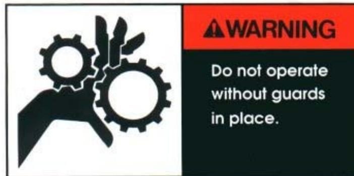
Figure 1-20 Guards-In-Place Warning Label (P/N 159062)
