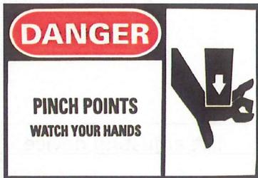
**Alerts you to the possibility of moving or rotating parts that could cause severe harm to appendages if caution is not use when operating the machinery. Keep hands clear when machine is running.**
