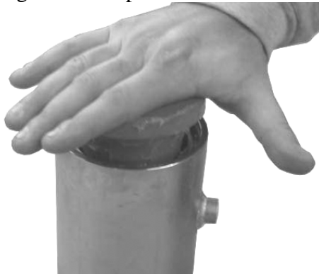
Figure 7-21. Push The Liner Into The Housing Until It Stops
