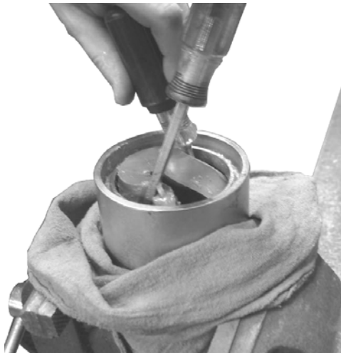
Figure 7-17. Using Screwdrivers To Squeeze The Pinch Valve Liner During Removal
