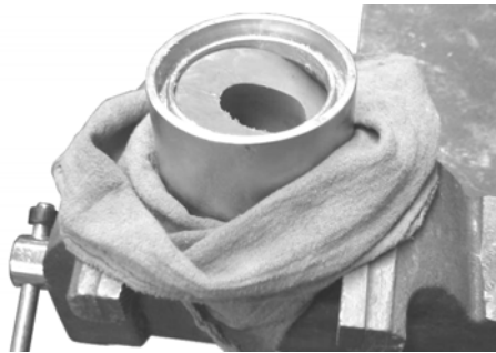
Figure 7-16. Wrap The Pinch Valve Cylinder Housing In A Shop Towel And Clamp It In A Vise
