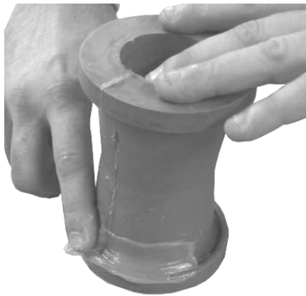
Figure 7-19. Application Of Silicone Lubricant to Lip Of Pinch Valve Liner
