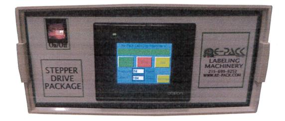
When you first turn the main power switch on it will take approximately 15 seconds for the PLC to do a self check and boot up. Once the PLC is fully powered up it will be in "RUN" mode and the screen shown below will appear.
