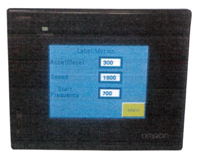
The feed of the label is controlled by a stepping motor. Each time the product sensor is triggered, the motor dispenses a label. Each time the label sensor sees the gap in between labels, the stepping motor stops label feed. You can make adjustments to the stepping motor by pressing the motor settings button.
