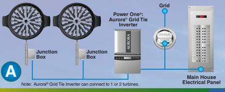
Grid Tie easy connection to utility -up to 2 tubines per Aurora® Inverter, no batteries required
