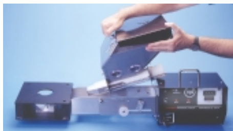
MCF Hopper being removed
