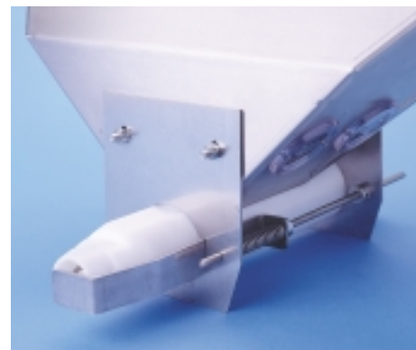
Pellet shutoff closeup
