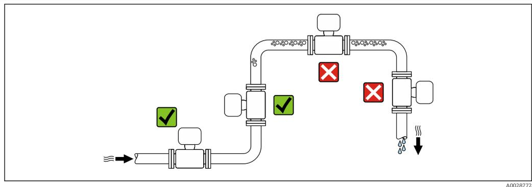
To prevent measuring errors arising from accumulation of gas bubbles in the measuring tube, avoid the following mounting locations in the pipe:
