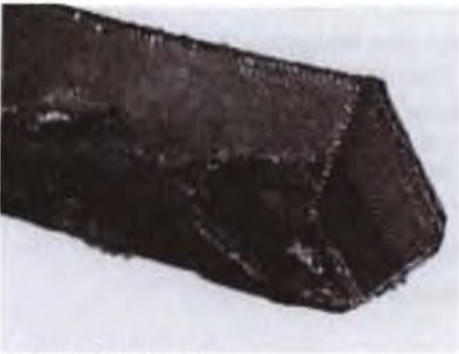
Cover Fabric Rupture
