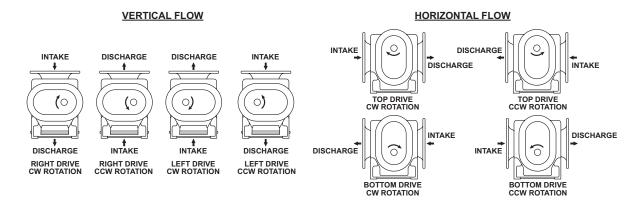
Figure 4-2 – Flow Direction by Rotation
