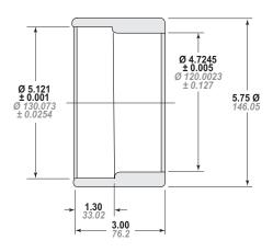
Figure 12-2 - Seal Installation Tool
