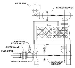
Figure 5-1 – Typical Blower Installation
