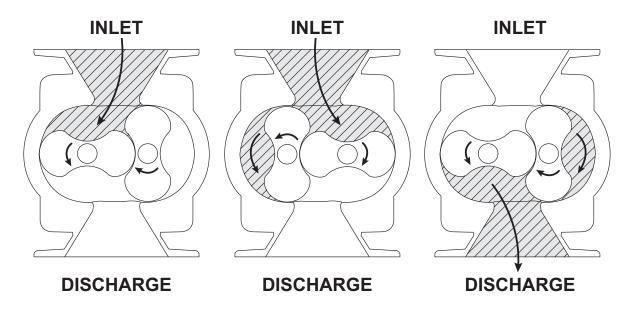
Figure 4-1 – General Operation Principle
