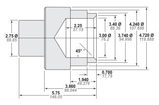
Figure 12-1 - Lab Seal Pressing Tool
