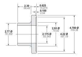
Figure 12-4 – Bearing Pressing Tool
