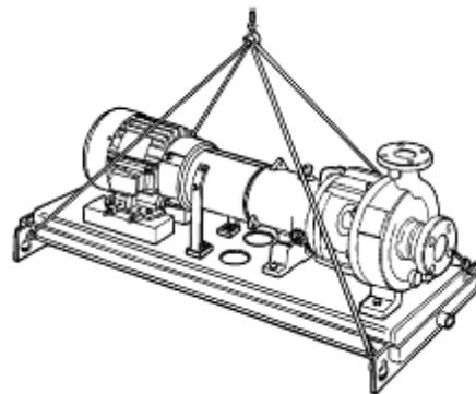
For other baseplates, sling around the pump discharge nozzle, and around the outboard end of the motor frame using choker hitches pulled tight. (Figure 2-4.) T5000 type bases should not be lifted with motor attached (i.e. pump and base only).
