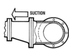
Start up strainers must be removed shortly before start up. When the pump is installed below the source of supply, a valve should be installed in the suction line to isolate the pump and permit pump inspection and maintenance. However, never place a valve directly on the suction nozzle of the pump.
