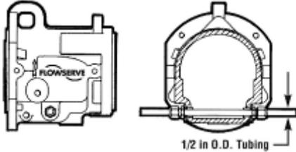
**4.6.6.5 Piping connection - support leg cooling for centerline mounting option**
