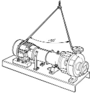
The sling should be positioned so the weight is not carried through the motor fan hood. Make sure the completion of the choker hitch on the discharge nozzle is toward the coupling end of the pump shaft as shown in figure 2-4.
