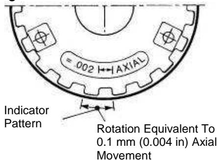
Determine how far to rotate the bearing carrier by dividing the desired impeller clearance by 0.1 mm (0.004 in.) (one indicator pattern). Tightening the set screws [6570.3] will cause the impeller to move 0.05 mm (0.002 in.) closer to the rear cover because of the internal looseness in the bearing carrier threads. This must be considered when setting the impeller clearance. Rotate the bearing carrier clockwise the required amount to get the desired clearance to the cover.
