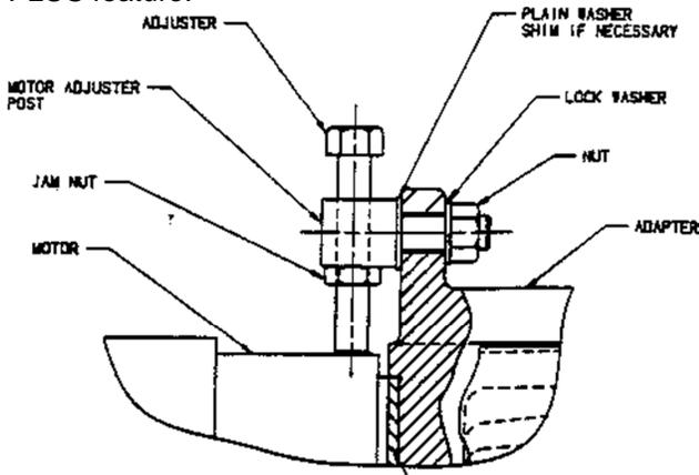
The motor mounting screws must be snug but not tight when attempting to adjust motor location. Depending on the size of motor it may be necessary to check the alignment with the motor fasteners tight. Corrections may be made until 0.002" TIR (or the desired) alignment is achieved. The adjusters, adjuster jam nuts and the motor fasteners should all be tightened. The indicator kit should be removed, the coupling and coupling guard properly installed
