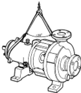
In-Line pumps: lift with two slings through the pump adapter on opposite sides of the shaft. (Figure 2-2.)
