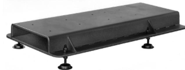
Baseplates intended for grouted installation are designed to use the grout as a stiffening member. Stilt mounted baseplates, on the other hand, are designed to provide their own rigidity. Therefore the designs of the two baseplates are usually different.
