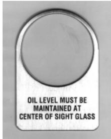
*“Oil level must be maintained at center of sight glass”.*
