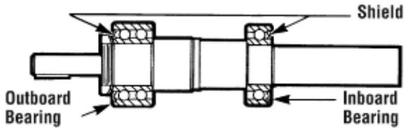
**Figure 5.9: In-line pump shield orientation**
