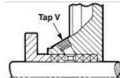
Grease lubrication, when compatible with the liquid being pumped, may be used. Again, introduced into tap V.
