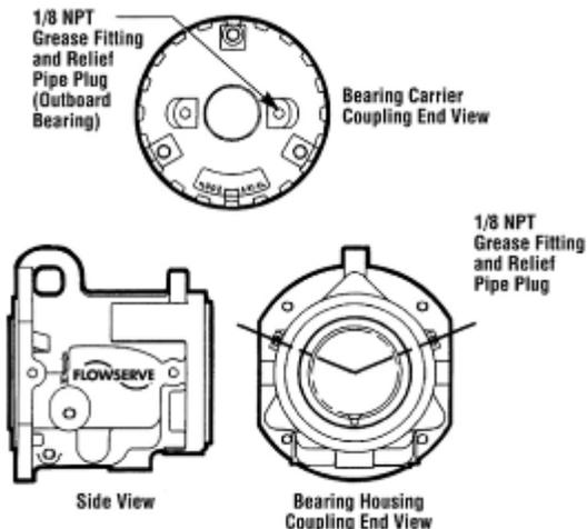
The amount of grease required for horizontal pumps is shown in figure 5.11
