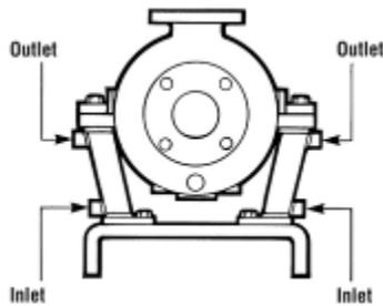
**4.6.6.6 Piping connection - heating/cooling fluid for jacketed cover/casing**
